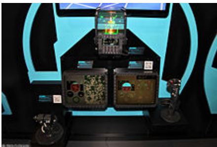
Su-35S cockpit layout: a head-up display , two multi-function liquid crystal displays, and a control stick with HOTAS
